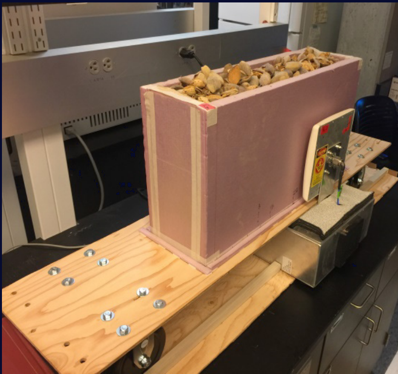
Microwave antenna with sample of in-hull almonds to measure kernel moisture content
