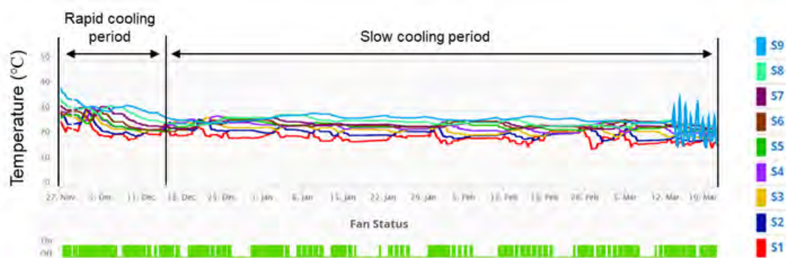
Figure 17. Example of multiple reheatings of grain (sensor S1 at bottom) during storage.
