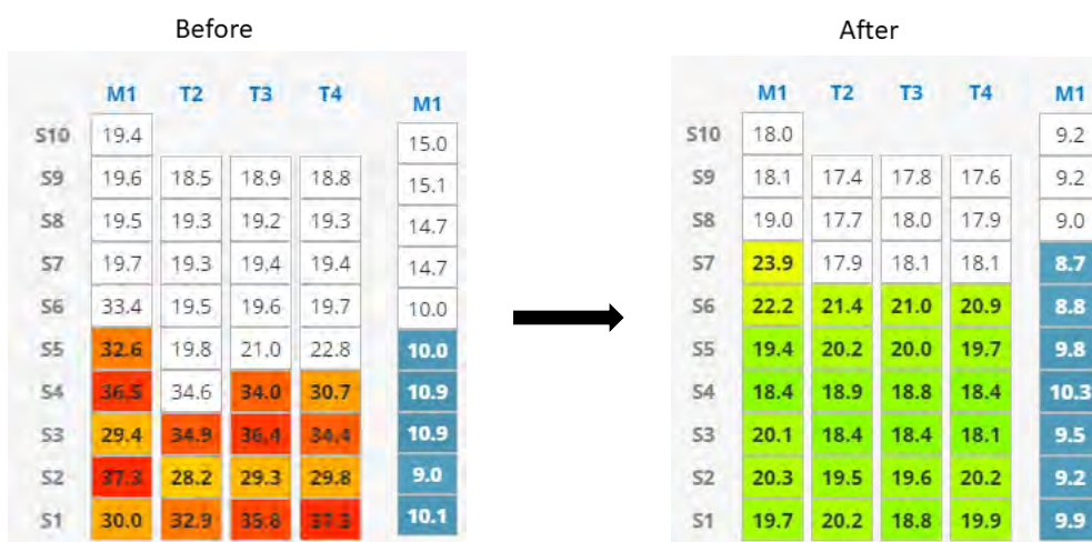
Figure 16c : Aeration cooling of 1,000 t white pained silo with 5 kW fan Barley = 140 fan hours from 5/12/20 to 12/12/20
