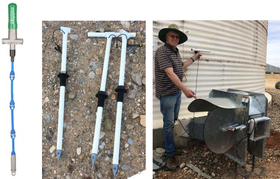
Figure 38. Example of silo sensors on a fixed cable (left), individual sensors fitted to removeable 1m long spears (centre) and spear inserted into silo above fan entry to silo (right).
